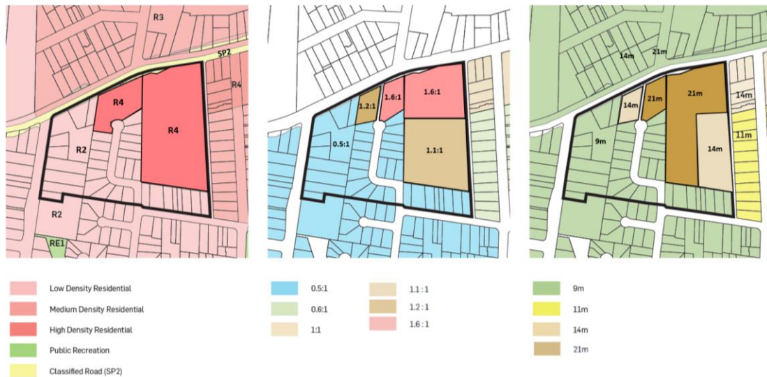
Figure 11 – Recommended planning controls for both planning proposals (remainder of block study area is subject to a future planning proposal)
